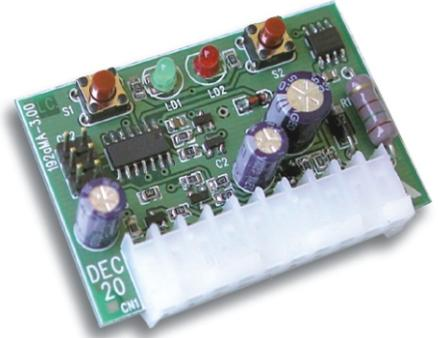
DEC20 is a twin channels decoder for BIRD antenna receiver and it's used for the installation on PCM1, PCM10F, PCM10S, PCM20 e PCM30 automation central units.
